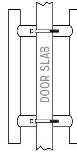
Back-to-back mounting features two door pulls which are connected through the door, each pull opposite the other.
